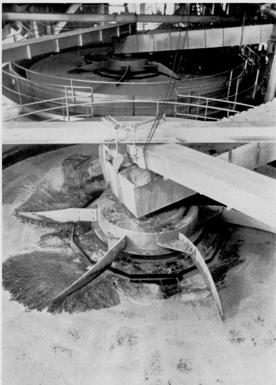
Fig. 4. — Primary I.H.C. — Cleaveland jigs of 25' diameter on Selangor N° 2 dredge (note skimmer with blades).
