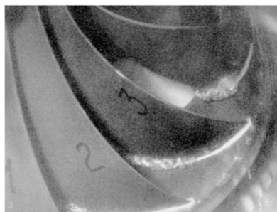
Fig. 3. — Leading edge cavitation in Francis machine.
