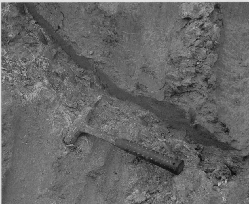
Fig. 5. — Active fault observed in weathering cover of Neocene sediments, 6 km SE of Laocai city.
