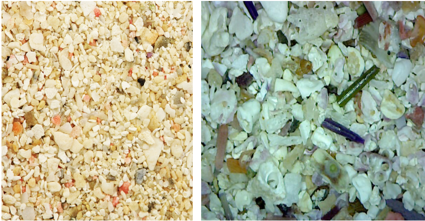
Fig. 8. — Silica sand (left) and carbonate sand (right).
