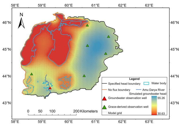
The discretized domain of the Modflow model and the simulated groundwater head. The Polygons surrounded by blue borders are specified head boundaries to simulate water body. The groundwater head is based on the simulation result of February 2005.
