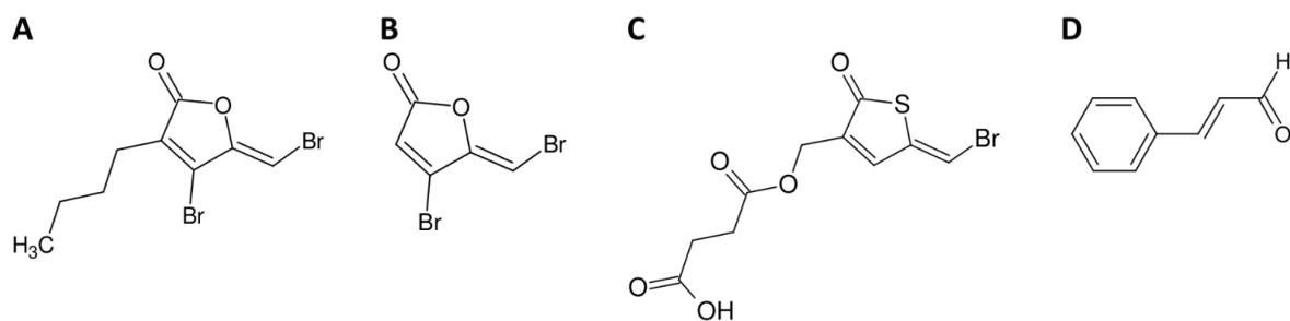
**Figure 4.** Chemical structure of quorum sensing inhibitors. (A) The natural furanone (5Z)-4-bromo-5-(bromomethylene)-3-butyl-2(5H)-furanone, produced by the red marine alga *Delisea pulchra*. (B) The synthetic derivative (5Z)-4-bromo-5-(bromomethylene)-2(5H)-furanone. (C) The brominated thiophenone (Z)-4-((5-(bromomethylene)-2-oxo-2,5-dihydrothiophen-3-yl)methoxy)-4-oxo-butanoic acid. (D) Cinnamaldehyde.
