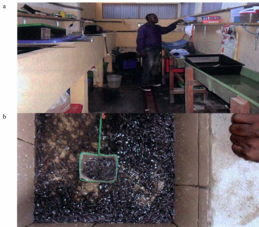
Fig. 7. — (a) Artisanal hatchery for catfish built by S. Mutambwe at M'Binza Pigeon, Kinshasa; and (b) full tank of African catfish fry of about 0.5 g.
